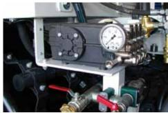
ESE 6 High-pressure water system inclusive of stainless steel hose reel High-pressure water system, integrated into the suction excavator, 10 m high-pressure hose, handheld spray gun with pointed spray nozzle for loosening the soil, wide-angled spray nozzle for washing operations and vehicle care, filling and overflow valves, 10 m water hose for filling the tank, 60 micrometer water filter hydraulic drive (Q = 20 l/min und p = 210 bar), water pressure ca. 200 bar.
