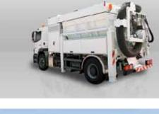
The RSP suction superstructure has been designed and optimized for specific uses on construction sites. A stainless steel drip edge helps reduce dirt accumulation during the emptying of liquid materials. The containers are built in different sizes to suit the different chassis sizes.
