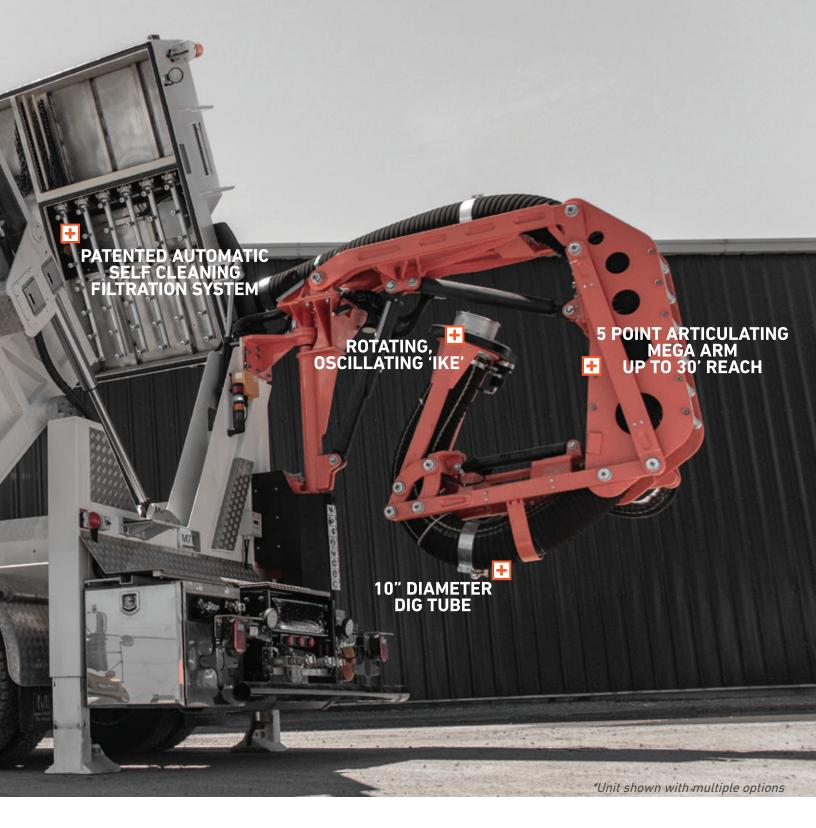
The innovative MTS Dino Series suction excavator is purpose-built for dry, from the ground up, to powerfully and safely excavate without the use of water.
